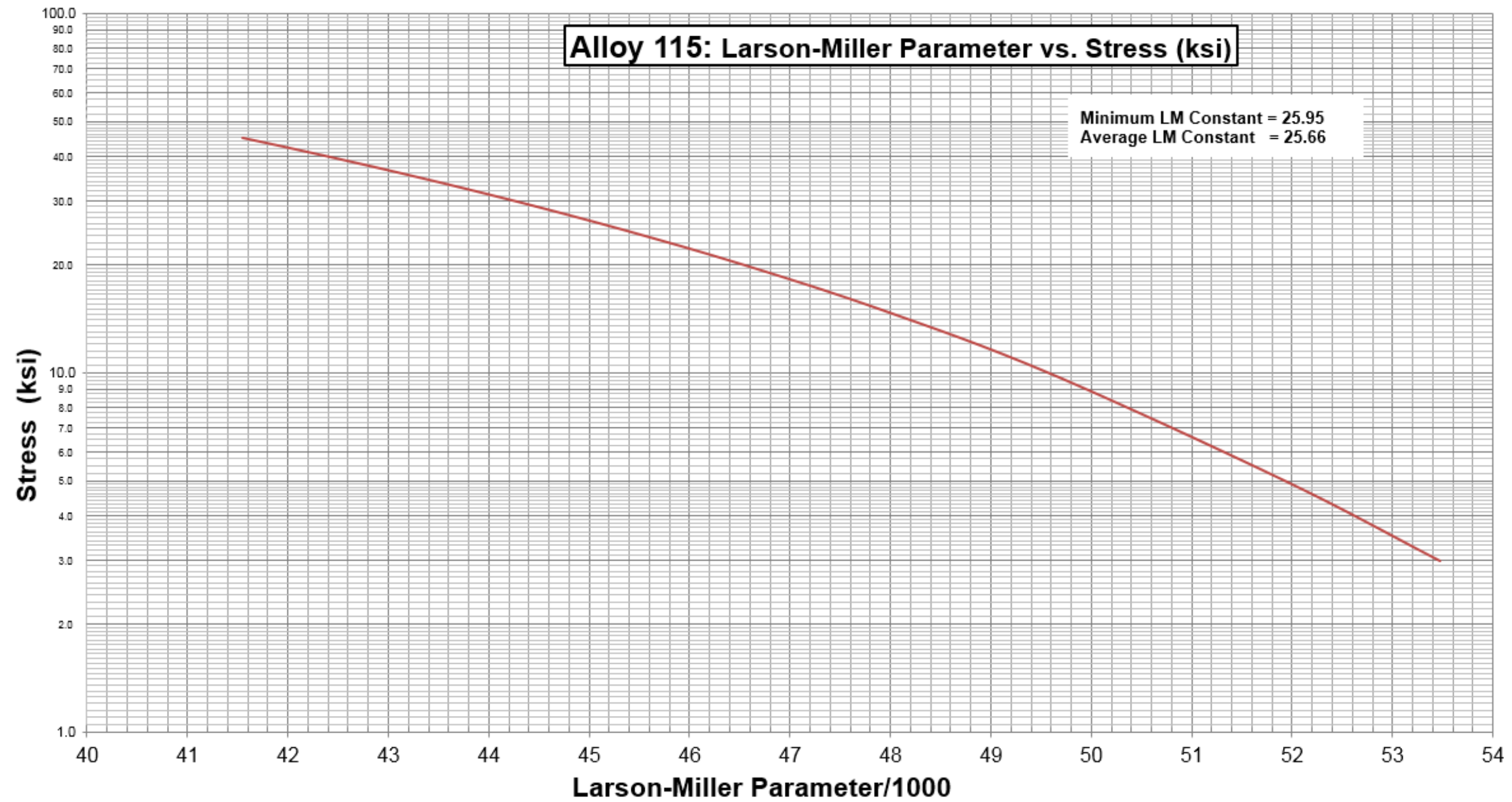
Figure F.36—Larson-Miller Parameter vs. Stress Curve (USC Units) for ferritic steel ASTM A213-T115 and A335-P115 10.5Cr-V Steels (Alloy 115)
